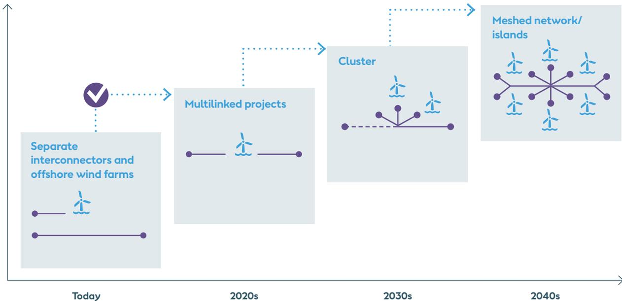
These cost-efficiencies can be even greater, if multilinked offshore wind farms are combined with optimised localisation of future power-to-X plants, as this leads to substantial system benefits and reduced transmission needs. Together, the required interconnector in 2050 can be reduced by 20%, compared to a scenario without multilinked wind farms and without redistribution of power-to-X products, the study suggests.
